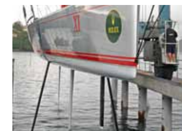
FOILS From left to right: starboard daggerboard, rudder, keel, forward centreboard, port daggerboard. The aperture for the lateral foil can just be seen on the starboard side of the hull. Note original position of the bobstay
